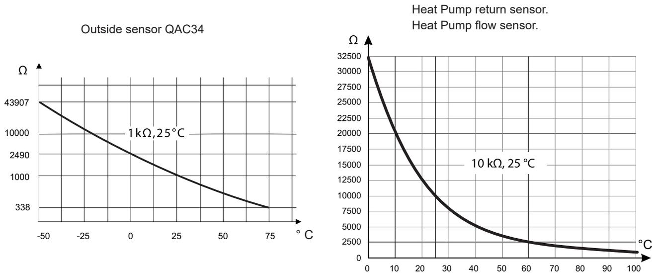
fig. 5 - Ohmic sensor values (Hydraulic unit)
