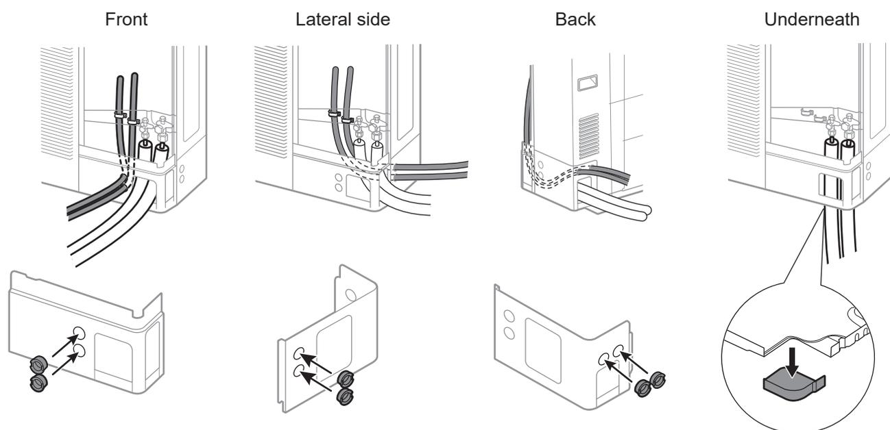
fig. 42 - Location of electrical cables and refrigeration connections to outdoor unit (Model 10)
