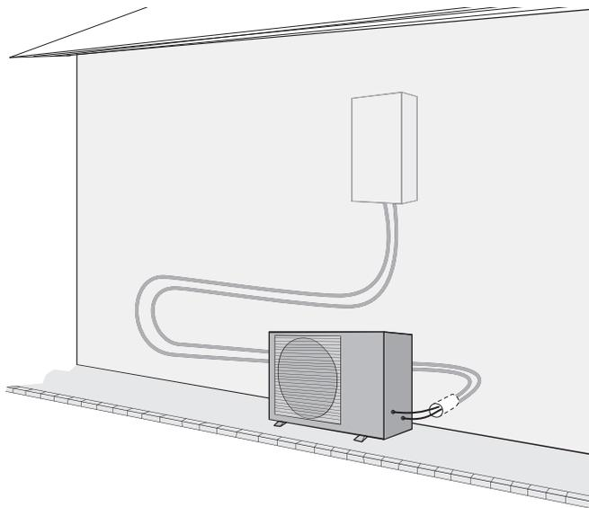
*fig. 12 - Recommended layout of refrigeration connections*
