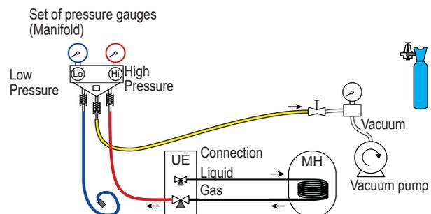
b) Switch off the vacuum pump, close the valve at the end of the service hose (yellow), connect this hose to the expansion valve on the nitrogen bottle, fill to 2 bar, close the hose's valve again,
