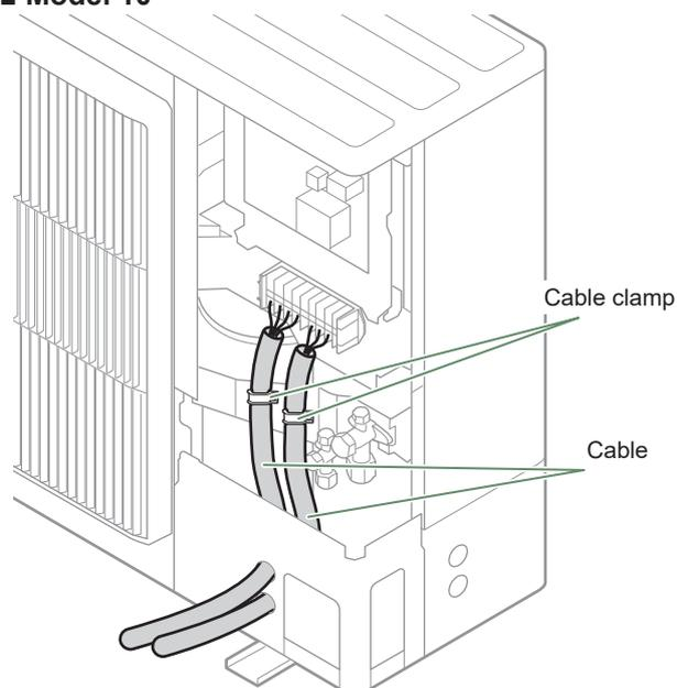
fig. 39 - Connections to outdoor unit's terminal block
