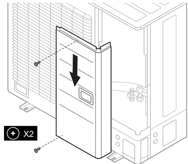
*fig. 14 - Open the outdoor unit model 10*
