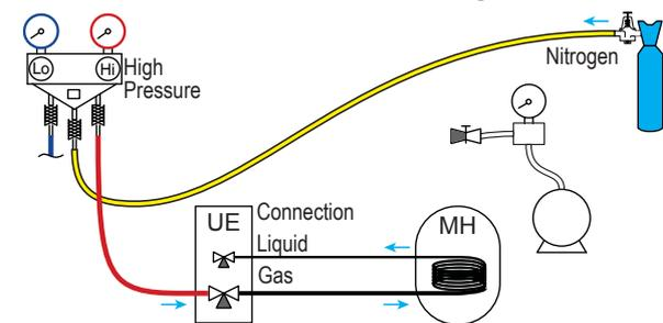
c) Connect this hose to the vacuum pump again, switch it on and slowly open the hose's valve.
