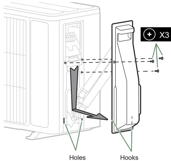
*fig. 13 - Open the outdoor unit model 5, 6 & 8*
