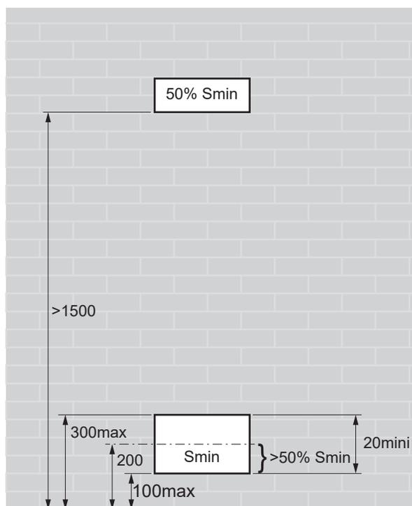
fig. 23 - Position of openings for ventilation
