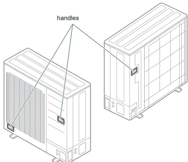
*fig. 15 - Transport of the outdoor unit model 10*
