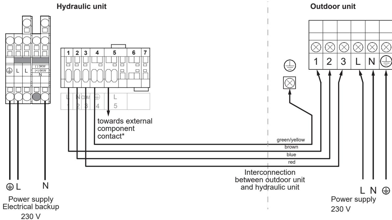
\* If the control device does not provide a potential-free contact, the contact must be relayed to create an equivalent wiring. In any case, refer to the instructions for the external components (power limiting device, electricity meter, etc.) to create the wiring.
