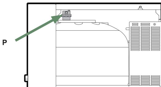
fig. 37 - Hydraulic unit automatic bleeder valve
